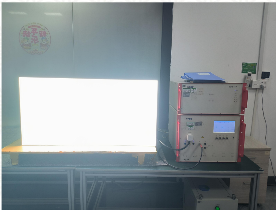
Figure 7: EFT/Surge/Dips Test Setup
